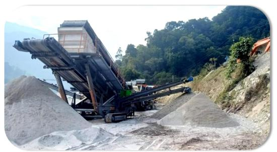
**SAEC** combines crushing, conveying and screening tasks, one machine can function as a complete production plant.
