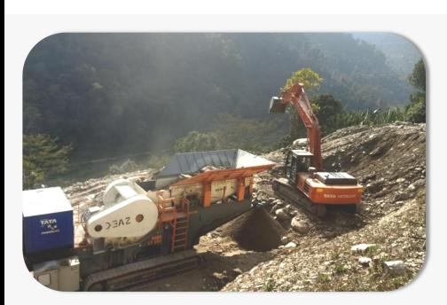
**SAEC** Series mobile crushers are widely used in aggregates production and recycling applications around the world. Thanks to track-mounted construction, LT machines are easy to move at a production site and transport between sites.
